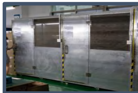
Wireless Shielding Room
